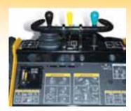
Transport and boom bucket motion are controlled by two ergonomically designed joysticks. The handgrip is positioned to help improve operator balance while on uneven terrain.
