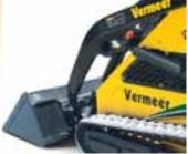
Curved loader arms lift up and away from the machine, providing better height and reach for loading and unloading. This also provides the clearance necessary to avoid damaging the front of the machine when using large-diameter augers and allows an operator to dump a bucket into the center of a one-ton truck.
