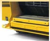
The ride-on unit comes with a spring-cushioned platform, keeping the operator out of mud and debris. At 14.5" (36.8 cm), it is high enough to enhance visibility while providing clearance for backing over curbs.
