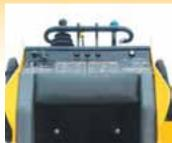
Cushions are positioned in front and on either side of the operator, increasing comfort and decreasing the chance of injury when driving over uneven terrain.
