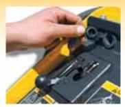
The standard auxiliary 12-volt power port lets operators power a temporary light kit or other attachments without having to tap into the unit's existing wire harness.
