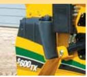
With a 15-gal (56.8 L) fuel tank, the S600 and S600TX boast the largest tank capacity in their class, eliminating the need for refueling during the typical workday. The 14-gal (53 L) hydraulic tank is also the largest of its class, enhancing the life of the hydrostatic system by increasing dwell time of the hydraulic fluid.
